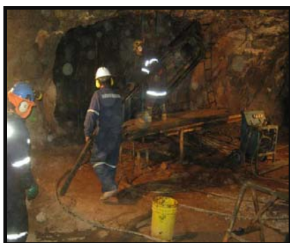
Underground diamond drilling
