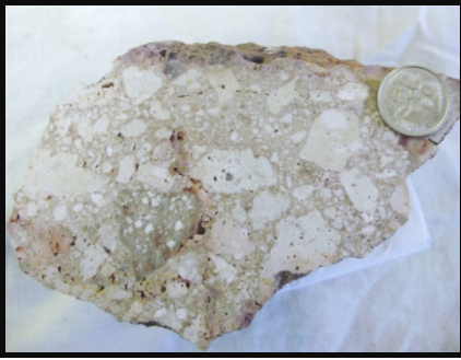
Mineralised lapilli tuff from the silver domain (mantos)
