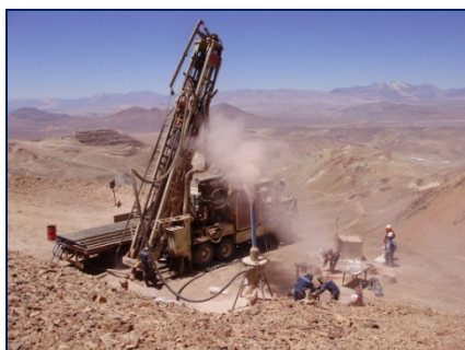
RC drilling at Arqueros Sur
