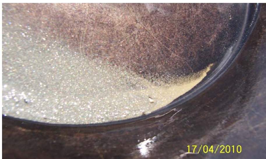
Figure 7. Photo Showing a Tail of Free Gold Panned from 192-193 Intercept in Hole 10EYRC0002 (fine yellow gold and silvery sulphides).
