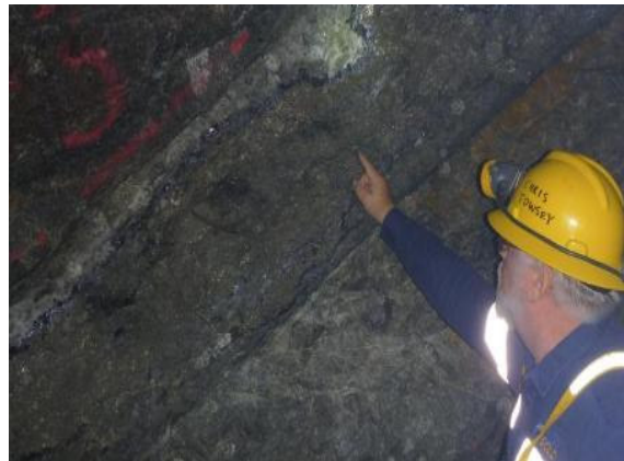
Mr Towsey, COO, underground inspecting the ore heading on the 855 level in the Sons of Freedom. The heading contains a gold vein 0.5 metre wide at grade of 326 grams per tonne gold.
