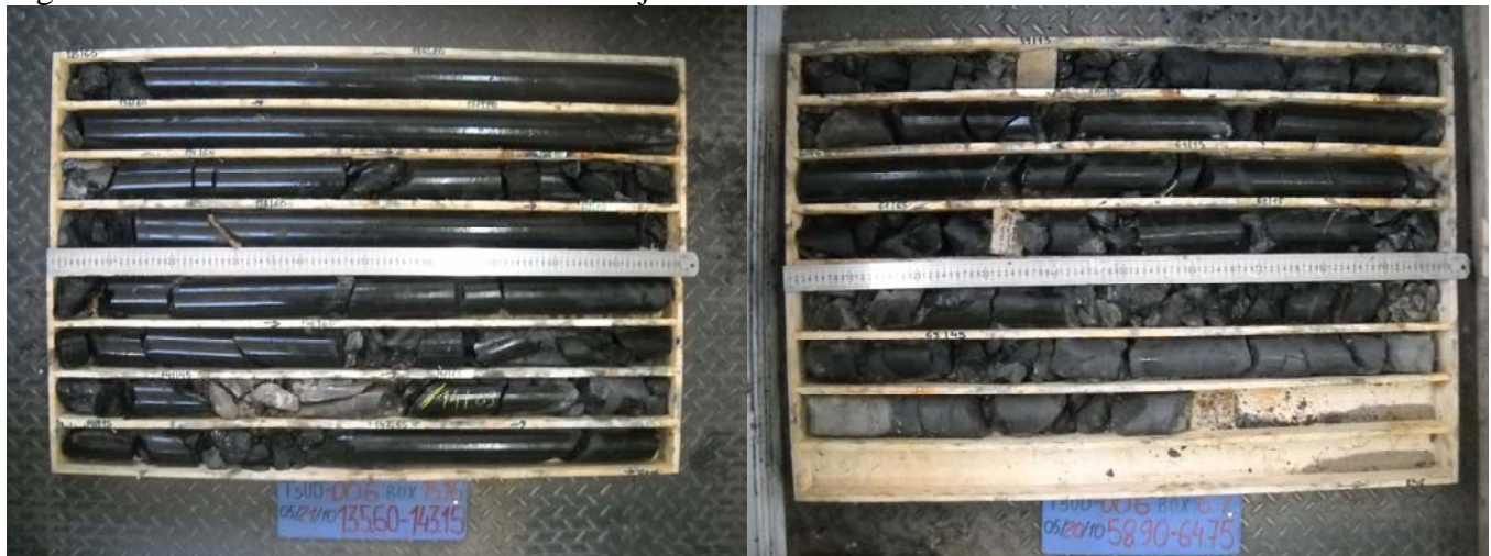
Figure 2. Drill core samples from the Drill Hole No.6
