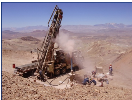
RC drilling at Arqueros Sur
