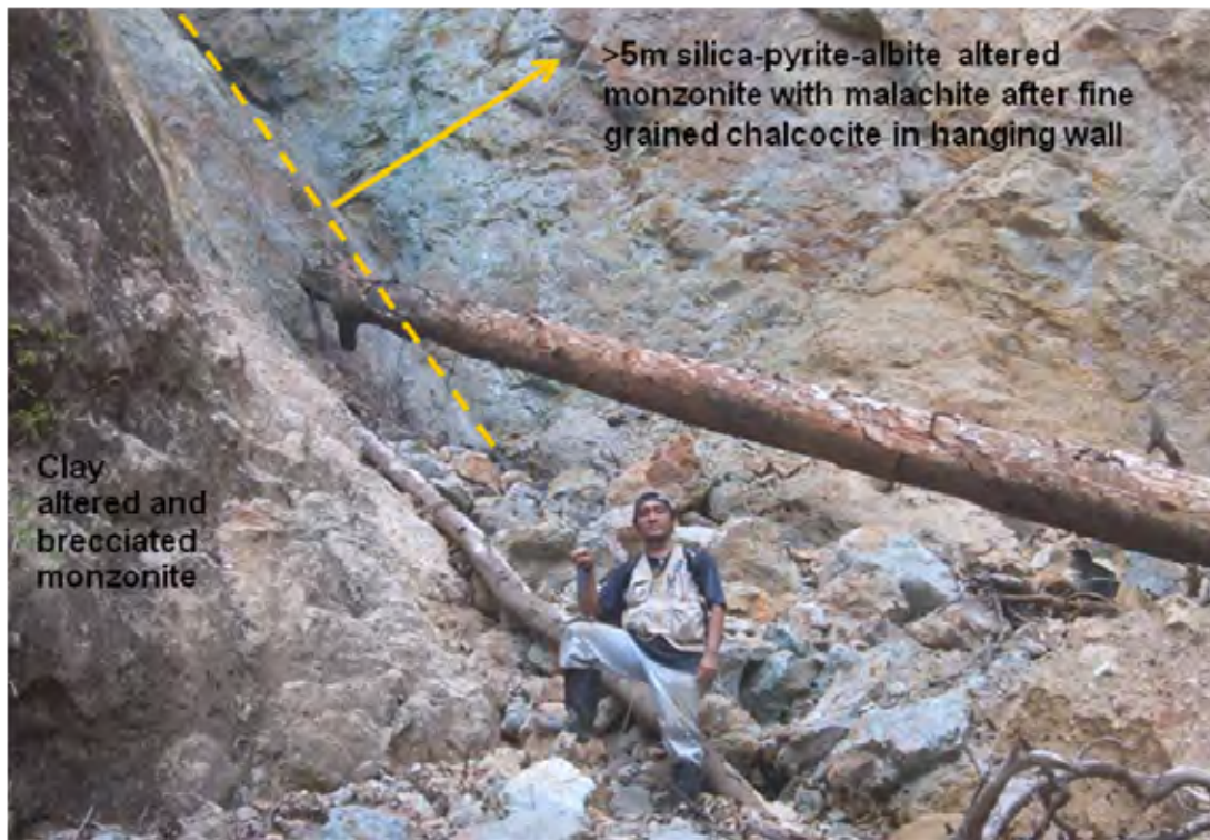
Photo 1. Exposed Rock Face Showing Abundant Copper Mineralisation (green malachite) at West Delta Prospect (assays pending)
