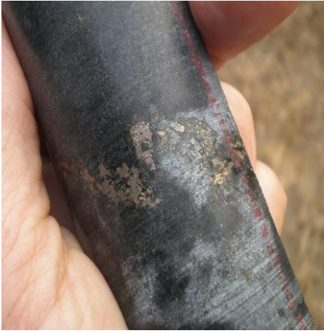
Sulphide mineralised drill core from drill hole TSD-01
