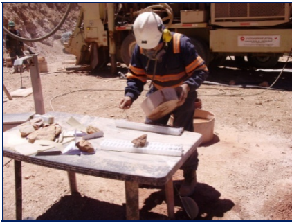
Driller preparing reverse circulation chips
