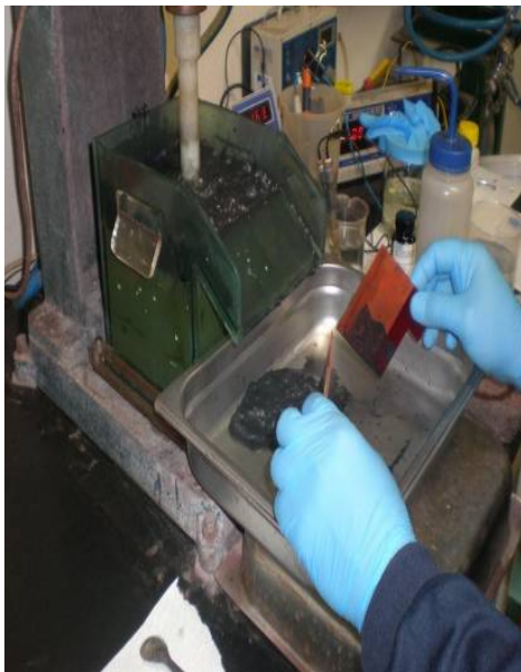
Copper sulphide flotation from the Antas South high grade zone at Rio Verde
