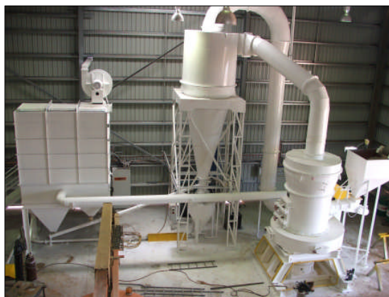
Grinding mill (50", 5 Roller Raymond Roller Mill)
