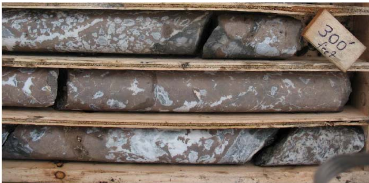
Massive, coarse grained zinc mineralisation intersected in DY-002, at the Darcy Zone, Yukon Base Metal Project.
